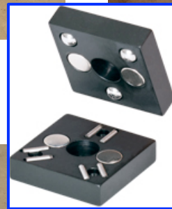
Ex-situ capillary holders for SAXS/WAXS (15 capillaries per holder)
