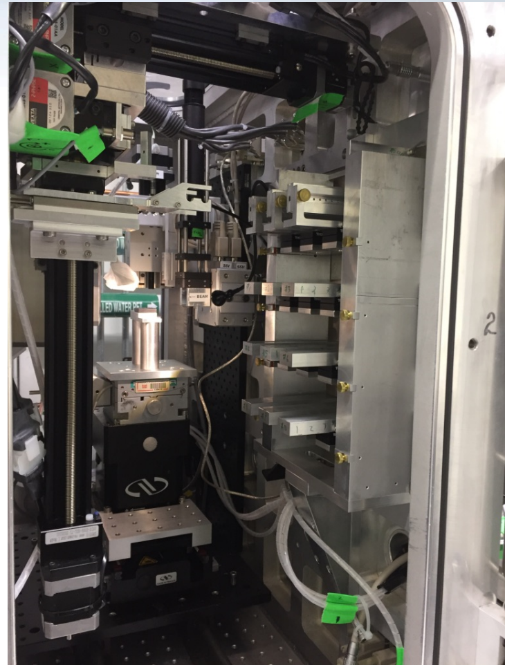
Sample exchanger (left) and garage (right) inside sample chamber
