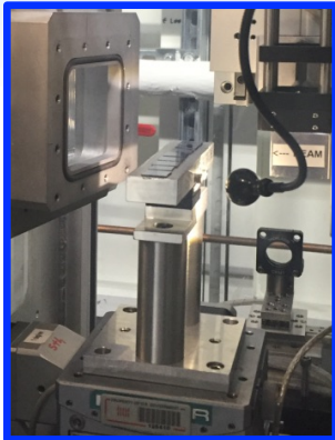
Ex-situ & in-situ T-annealing thin-film bar Sample rotation/mapping (CD-SAXS, GISAXS tomo)
