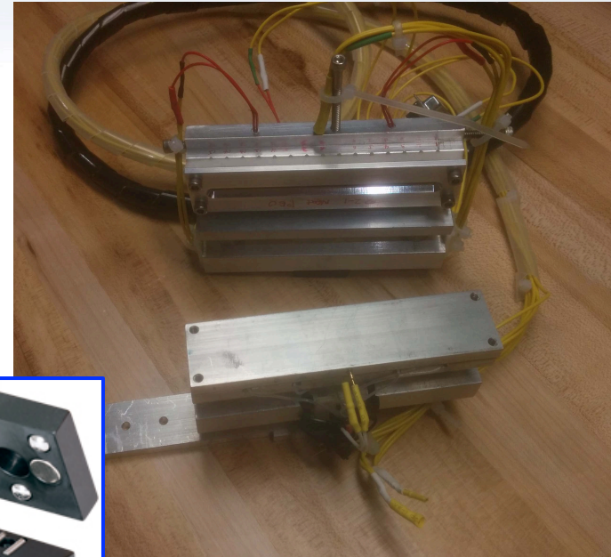
In-situ thermal annealing versions of capillary holders (top, tested to 80 °C in air) and thin-film substrate holders (bottom, tested to 220 °C in vacuum).
